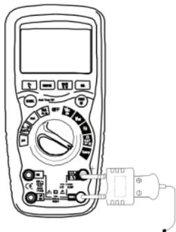
**NOTE:** The temperature probe is fitted with a type K mini connector. A mini connector to banana connector adaptor is supplied for connection to the input banana jacks.
